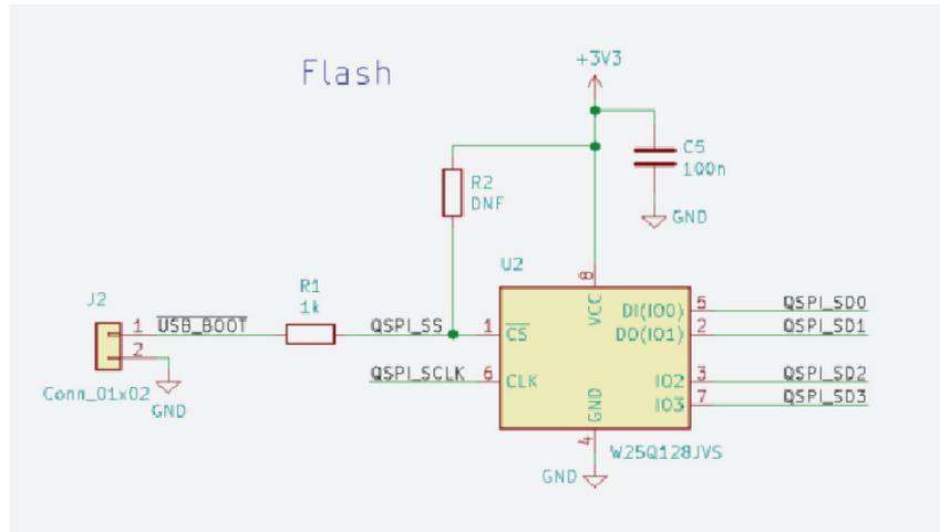
In order to be able to store program code which RP2040 can boot and run from, we need to use a flash memory, specifically, a quad SPI flash memory. The device chosen here is an *W25Q128JVS* device (**U2** in Figure 7), which is a 128Mbit chip (16Mbyte). This is the largest memory size that RP2040 can support. If your particular application doesn't need as much storage, then a smaller, cheaper memory could be used instead.
