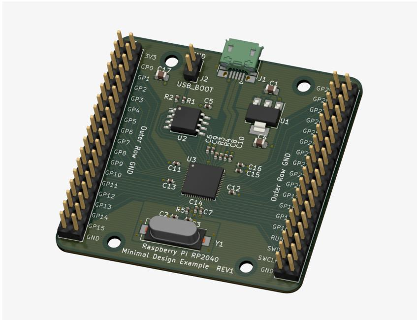
This minimal design example is intended to demonstrate how you can get started with your own RP2040 based PCB designs. It consists of very nearly the minimum amount of circuitry required to make a functional design that can run your code. Schematics and layout files are available for KiCad at <https://datasheets.raspberrypi.org/rp2040/Minimal-KiCAD.zip>. KiCad is a free, open source suite of tools for designing PCBs and can be found at <https://kicad.org/>.
